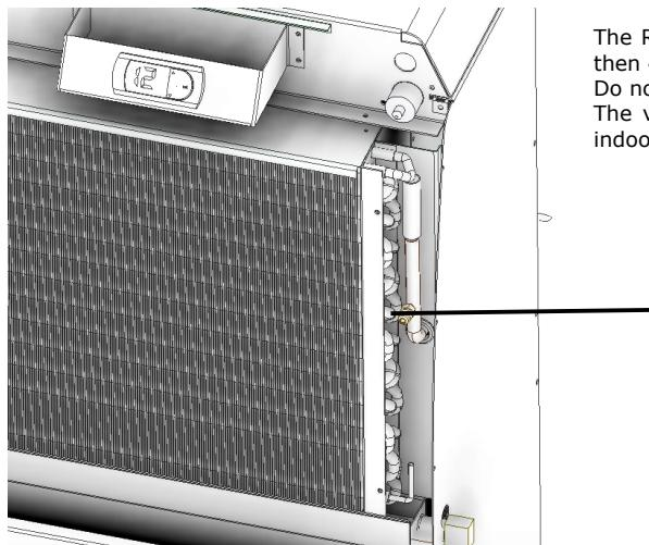
The R407C load must be 1kg up to a length of 8m, then 48g per meter.
